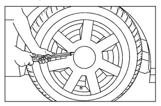
For models having aluminum wheels with a center wheel cover, use the flat end of the wheel wrench to gently pry the wheel covers off. Be careful not to scratch the aluminum wheel edge and do not try to remove it with your hands. Then loosen the wheel nuts with the wheel wrench. Do not remove them yet.
